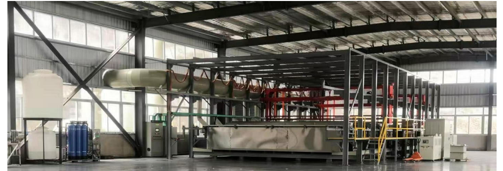
Surface treatment production line Micro-arc oxidation, passivation, electrophoresis, electroplating, powder spraying, and other coatings
